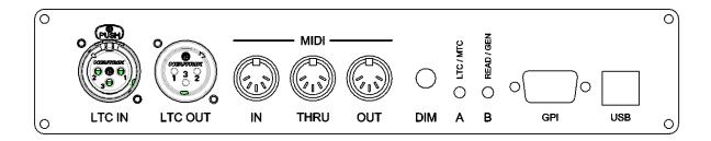
**LTC IN** – Balanced XLR input for LTC SMPTE signal when in reader mode.
