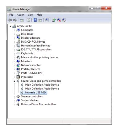
Windows 7/8/10 will detect the device and attempt to install it a standard USB MIDI device. It may connect to the internet to determine whether there is a driver to use other than the standard MIDI driver, but will be satisfied to use the standard class compliant driver.
